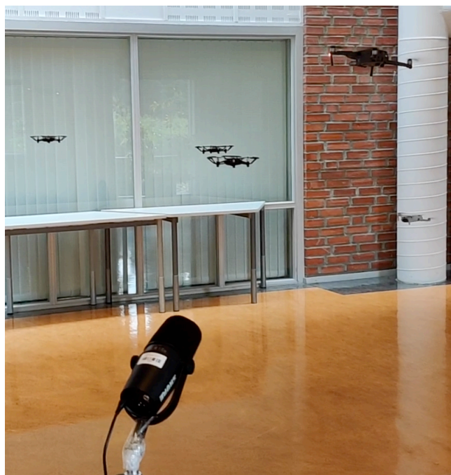
Figure D.3: Capturing acoustic signals for a 5 UAV scenario.
