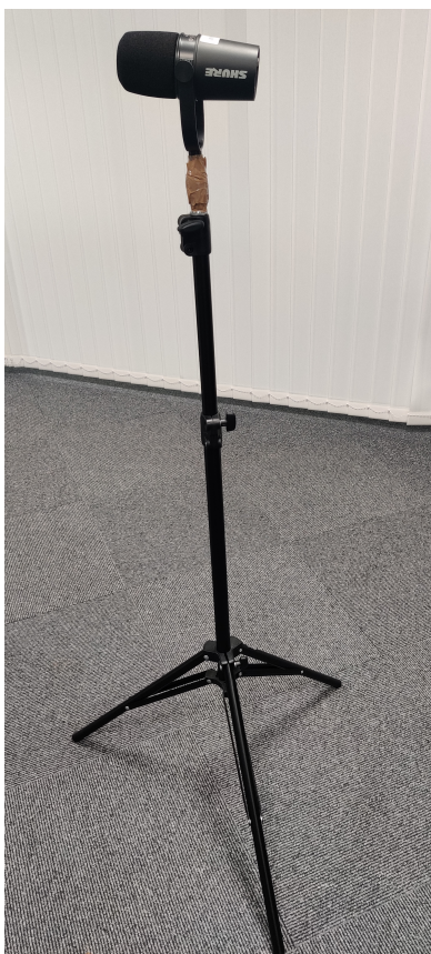
Figure D.2: Shure MV7 setup used for measuring the UAV acoustic signals
