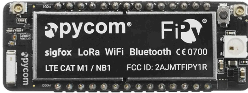
Figure 4.1: Pycom communication module.
