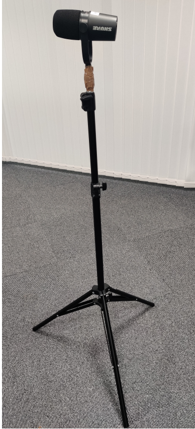
Figure 3.8: Shure MV7 mounted on a tripod to measure UAV acoustic signals [12].
