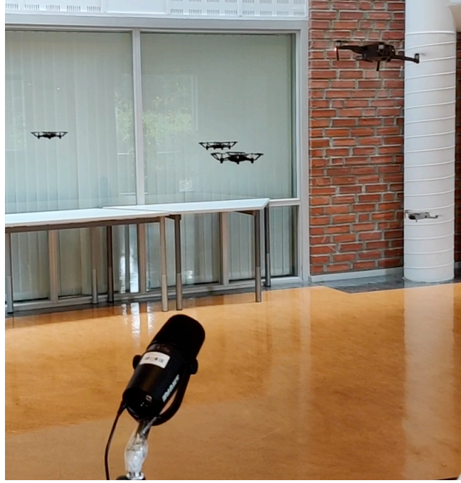
Figure 3.9: Recording UAV acoustic signals for a scenario with 5 UAVs [12].
