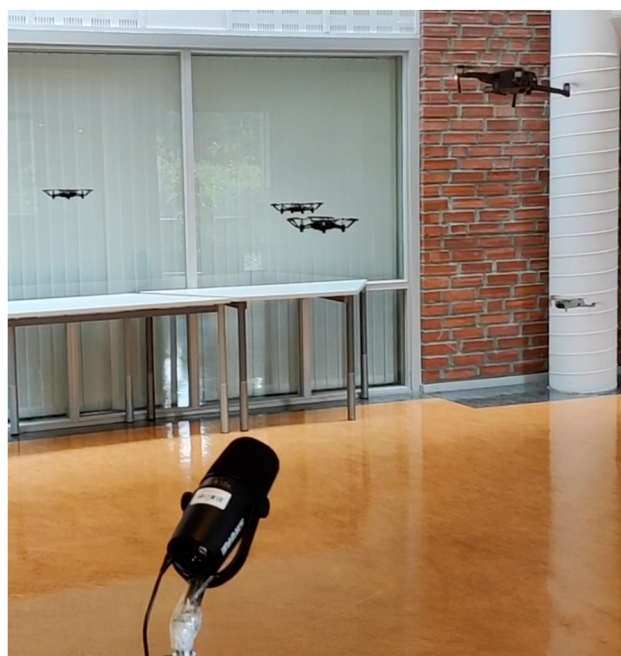
FIG. 3. (Color online) Capturing acoustic signals for a five-UAV scenario.
