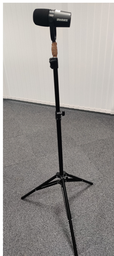
FIG. 2. (Color online) Shure MV7 setup used for measuring the UAV acoustic signals.
