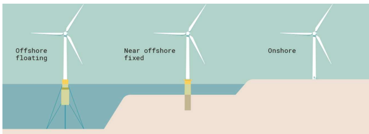
Figure 2: Schematic representation of offshore floating, offshore fixed and onshore wind turbines (Nord-Lock, 2020)
