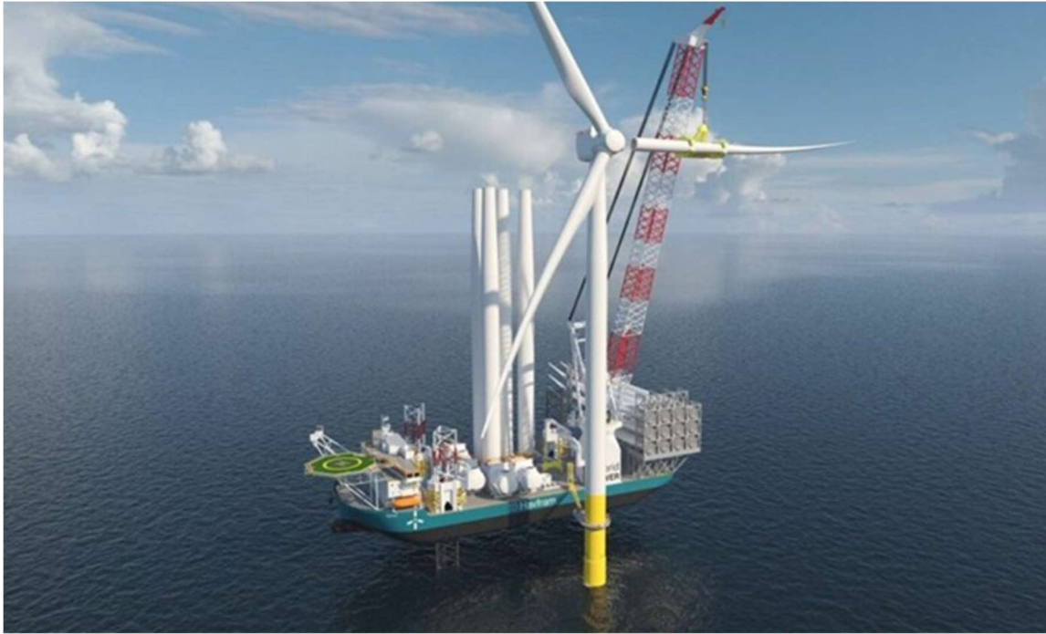
Figure 4: New WTIV Design by Havfram (Splash, 2023)
