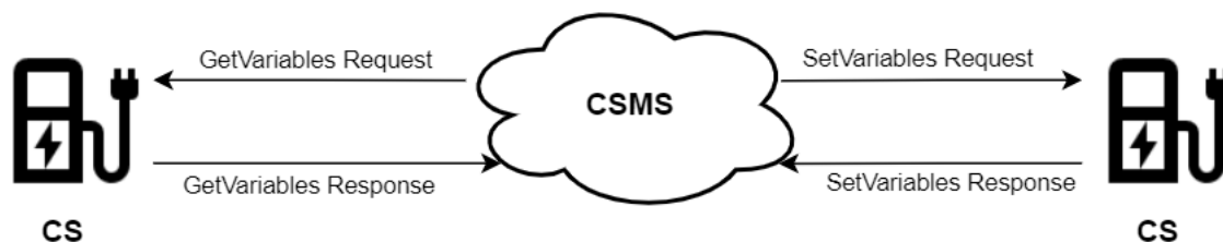
Figure 2.6: OCPP client server architecture
