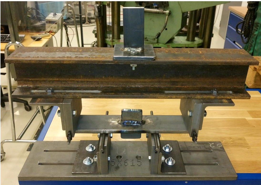
FIGURE B2. Test setup bending loading mode
