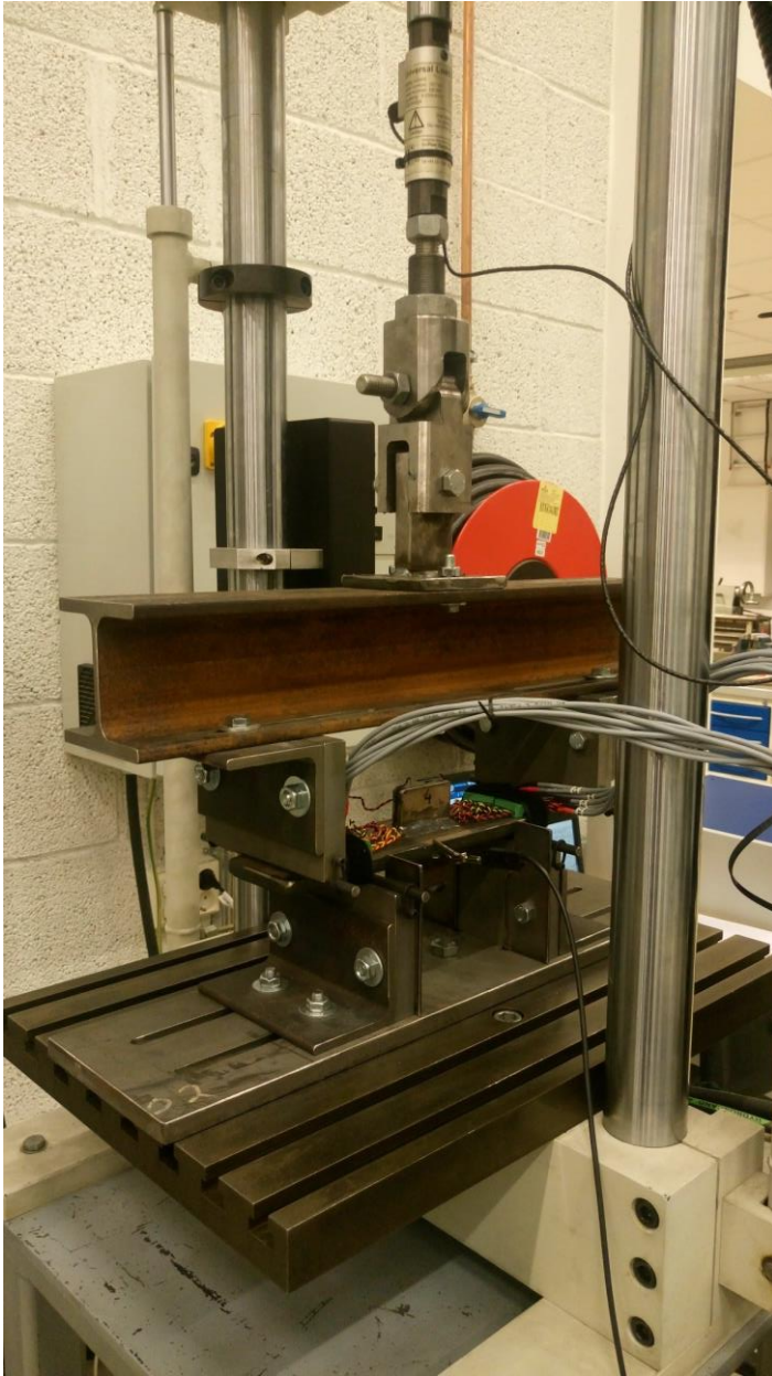
Figure A.4. Pusher on double hinge to balance the load (uniform loading on both ends)
