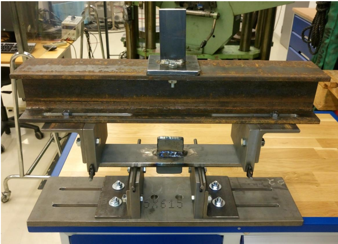
Figure A.3. Loading frame for 4-point bending
