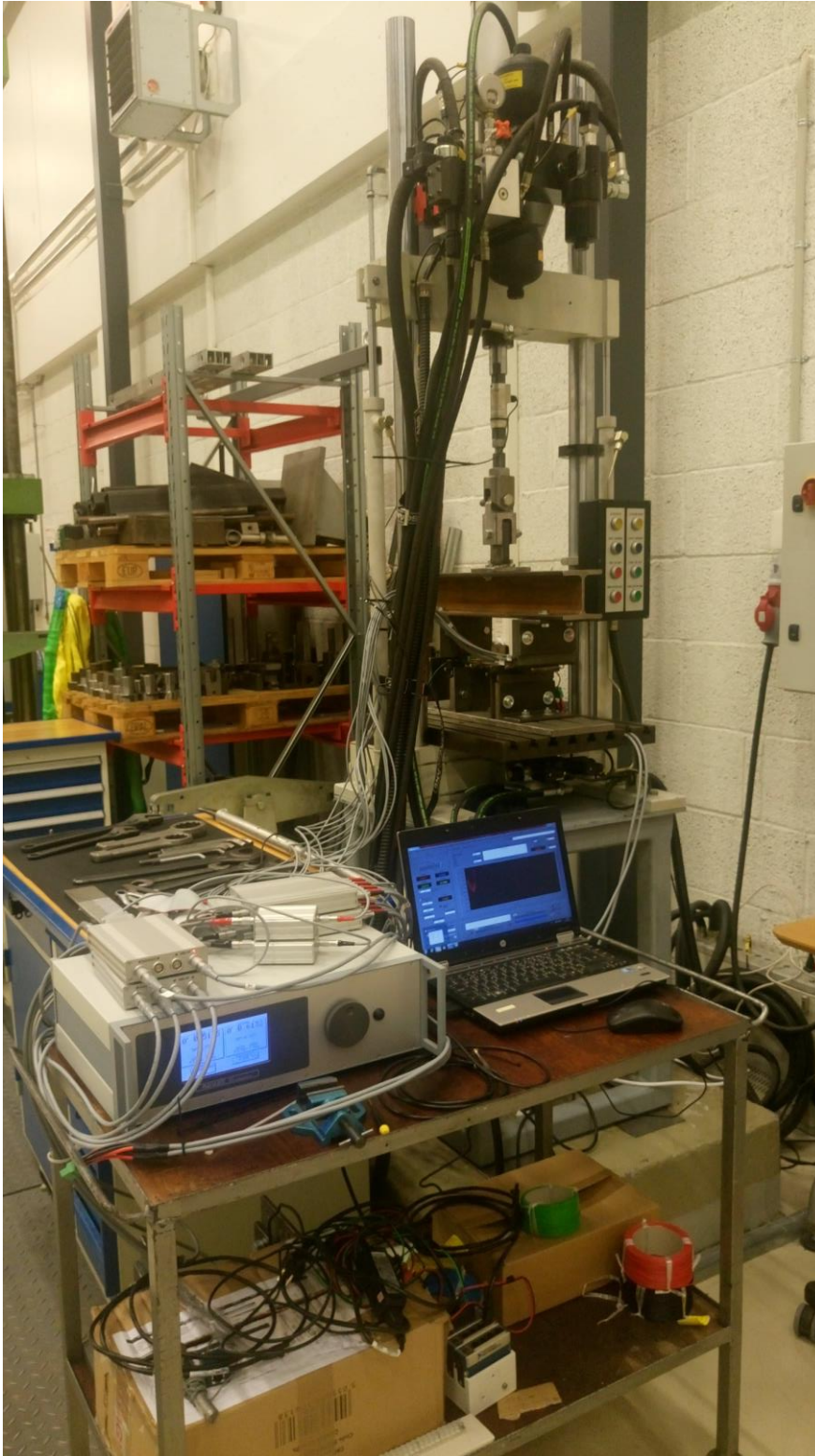
Figure A.2. Si-Plan fatigue testing machine with the assembled test rig
