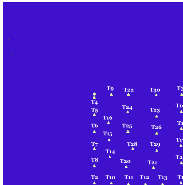
Figure 5.5: The 6 \text{ MW}/\text{km}^2 capacity density wind farm with 30 turbines of 5 MW.
