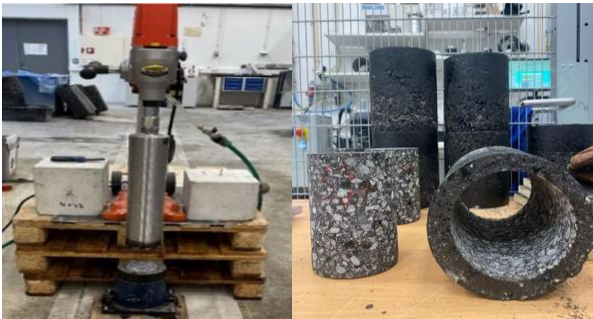
FIGURE 5.6: BORING AND CUTTING TO REQUIRED SAMPLE HEIGHT.
