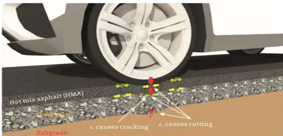
FIGURE 3.3: STRESS FORMATION IN AC LAYER DUE TO TIRE LOADING [59]
