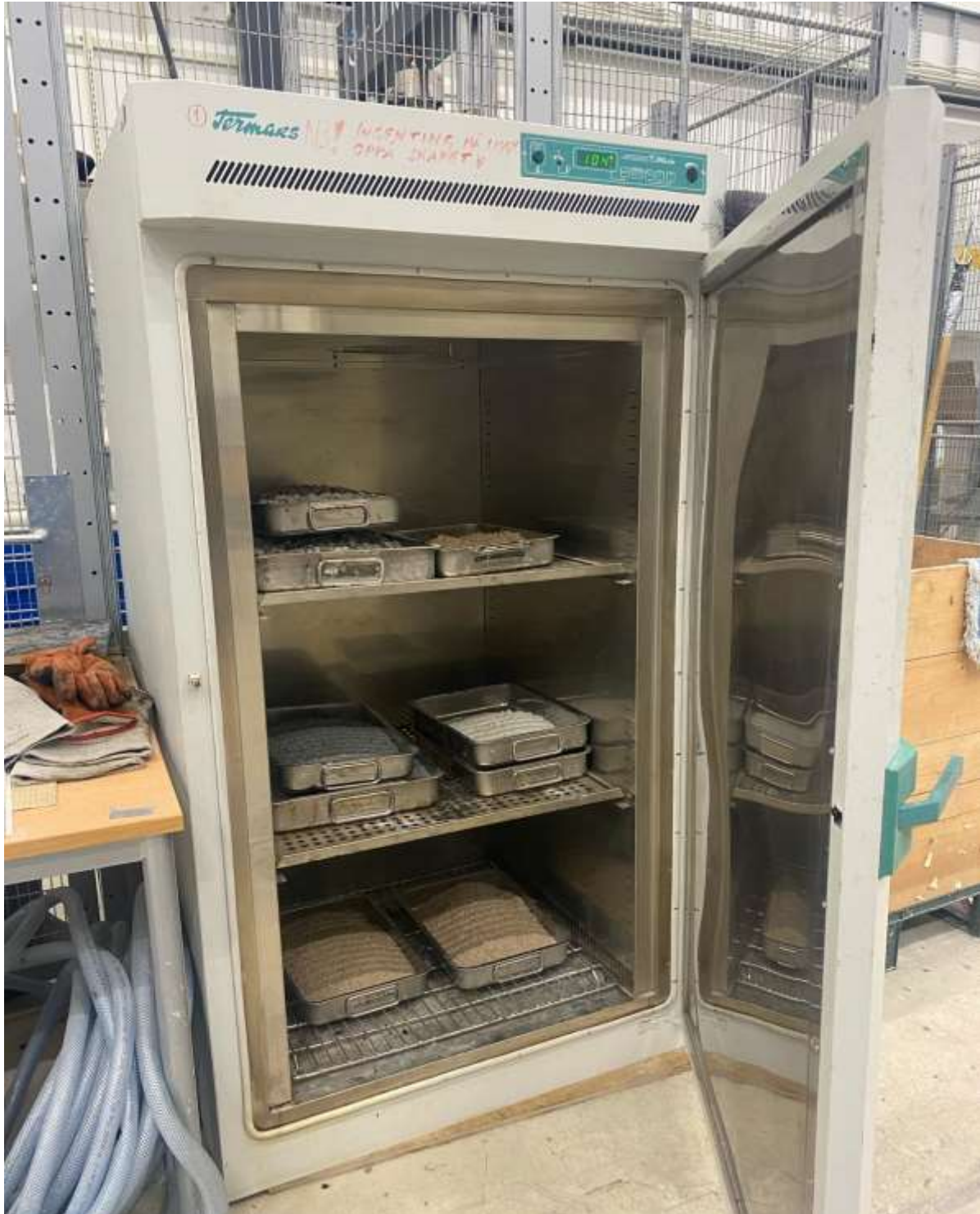
FIGURE 5.3: HEATING UP THE AGGREGATES BEFORE MIXING IN 110 °C FOR 24 HOURS.
