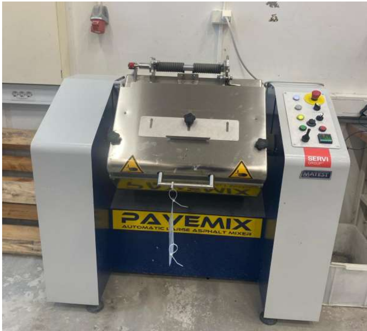
FIGURE 5.2: THE PAVE-MIX MIXER USED TO MIX THE HMA SAMPLES.
