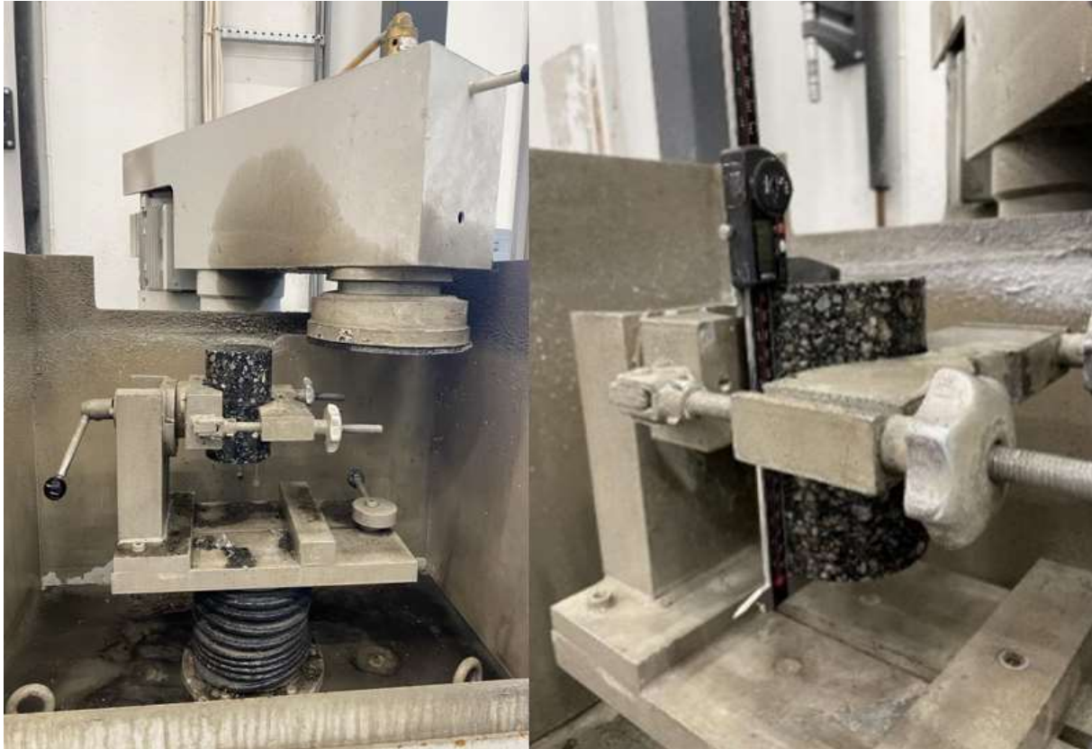
FIGURE 5.7: CUTTING AND SLIPPING TO REQUIRED SAMPLE HEIGHT
