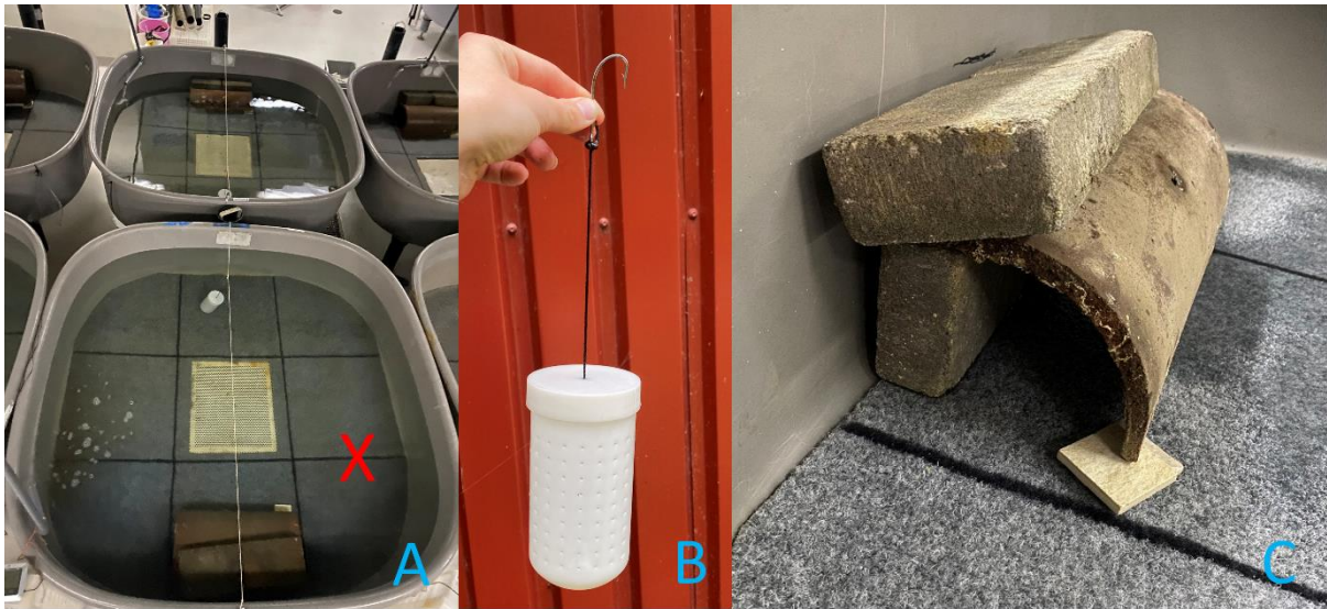
Figure 5 Picture A: Tank set up with both shelter and food box in the tanks, the red x marks where lobsters were put in the tank, facing away from the shelter, Picture B: The food box, Picture C: The shelter.
