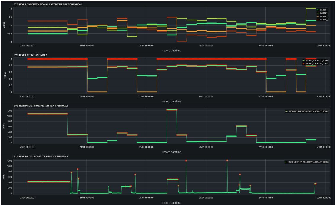
Figure 7.7: The DESMOD dashboard HEngCCM AD prediction using trained deep learning CGVAE model (see Section 4.1): a) sensor-level AD report summary, and b) system-level AD report.
