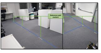
**FIGURE 8.** Left side and Right side of the area used for the experiments and reference path markers. The path in "T" shape to be followed by the target objects is partially shown in the picture in blue dashed lines. The sensor can be seen in bottom right with a distance of 1.5 m from each line of the path and remains static as the targe object moves through the path.
