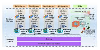
**FIGURE 3.** General architecture: Different pipelines with distributed nodes across two embedded devices. Data from cameras and LiDAR are preprocessed separately at a interface module and sent asynchronously to be fused at a fusion module.
