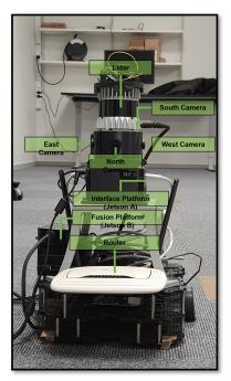
**FIGURE 6.** Proposed experimental setup. The mounting remains static and is placed on a suspended base for the experiments.
