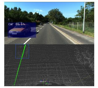
**FIGURE 16.** Illustration of experiments performed on KITTI-360 dataset [46]. The green line below represents the track of the car detected in the top image, displayed in the ego-vehicle coordinate frame.
