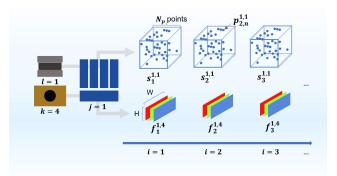
**FIGURE 1.** Illustration of the convention adopted. In the example, camera k = 4 and LiDAR l = 1 are connected to device j = 1, sending frames sequentially.
