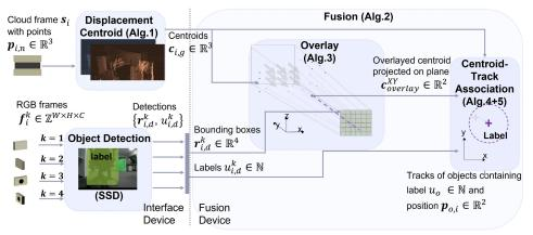
**FIGURE 4.** Data flow and algorithms. Cluster centroids are obtained from displacement in point clouds (Alg. 1). For each camera, bounding boxes and labels are obtained for every detection (Subsec. IV-C). After an approximate synchronization is performed (Alg. 2), the closest centroid overlayed by a bounding box is projected in the ground plane (Alg. 3) and can create or update tracks (Alg. 4). Non-overlayed centroids can also be used to update nearby existing tracks (Alg. 5).
