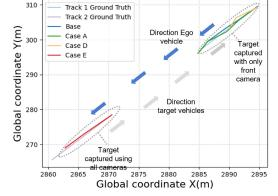
**FIGURE 17.** Localization of two vehicles captured using different cases and their track ground truths on KITTI-360 dataset [46] (Cases B, C ommitted for brevity). An additional car was only detected in Case E due to the extra cameras that captured it in lateral view.
