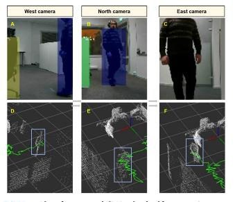
**FIGURE 11.** View of cameras and LiDAR point cloud for person. Camera images (A,B,C) with the respective point cloud correspondence (D,E,F) for person as object of interest. Detection occurring in both west (A) and north (B) cameras overlaying centroids for updating the track. East camera (C) without detection and only centroid is used for update.
