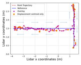
FIGURE 12. Trajectory corresponding to a person walking over the reference path. The arrows indicate the sequence of the trajectory and different symbols indicate point updates from overlayed (star) and non-overlayed centroids (circles) using for updating the track.
