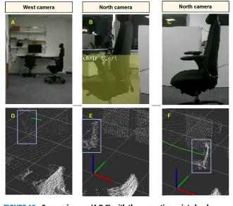
FIGURE 13. Camera images (A,B,C) with the respective point cloud correspondence (D,E,F) for a chair as object of interest. A: Even though the object can be seen from east camera, no detection occurs and the non-overlayed centroid updates the track. B: Detection occurs in north camera and centroid is overlayed. C: Detection fails again for north camera and centroid is not overlayed.
