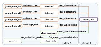
FIGURE 7. Software architecture. Arrows represent messages exchanged in a publisher-subscriber scheme.
