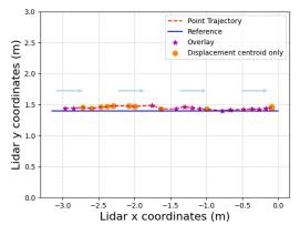
FIGURE 14. Trajectory corresponding to a chair being towed over the reference path. The arrows indicate the sequence of the trajectory and different symbols indicate point updates from overlayed and non-overlayed centroids used for updating the track.
