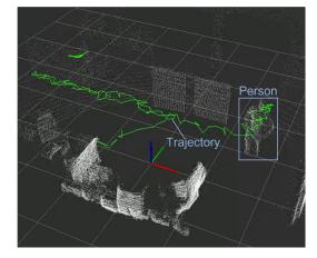
**FIGURE 10.** Trajectory of the reference point (geen lines) along with point cloud obtained through Alg. 1-5. The coordinate system is defined by the LiDAR on the setup, as illustrated by the red, green and blue arrows.
