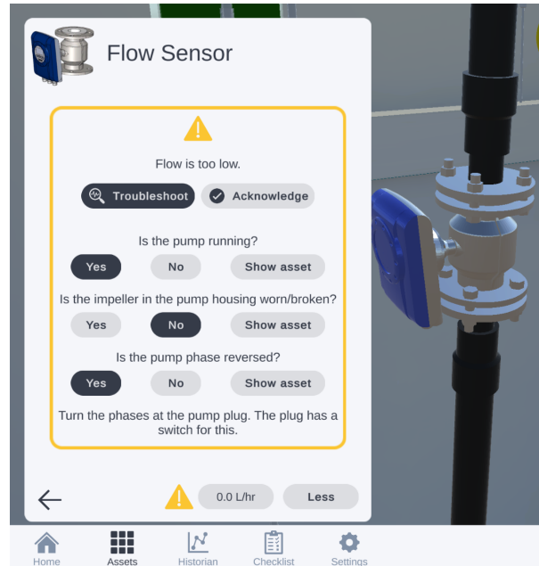
Figure 6. Troubleshooting guide for the flow sensor.
