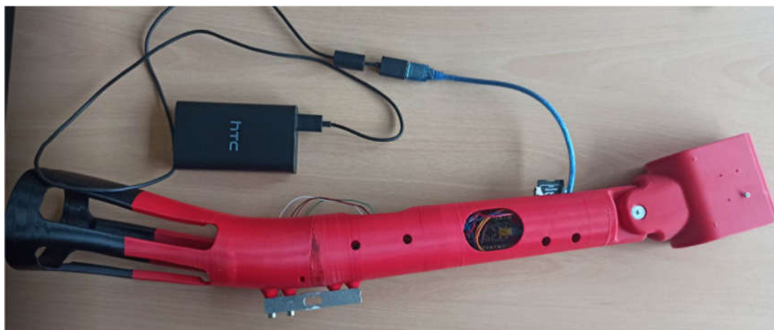
Figure 18. Prosthesis during laboratory tests with power source connected.
