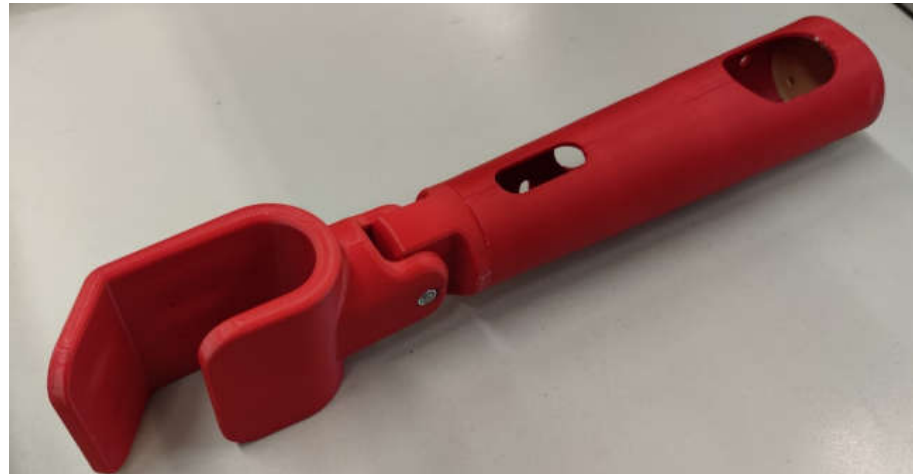
Figure 24. Assembled prosthesis forearm and end effector.
