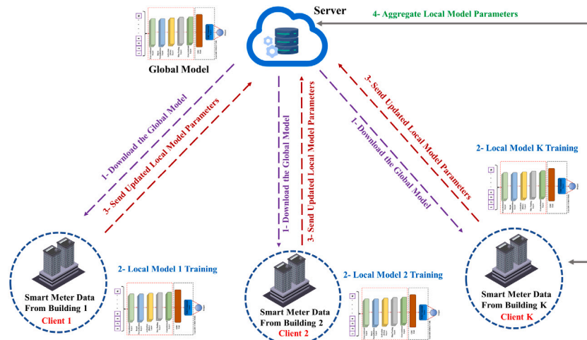
Fig. 6. Architecture of the Cross-Silo Federated Learning (FL) setup.
