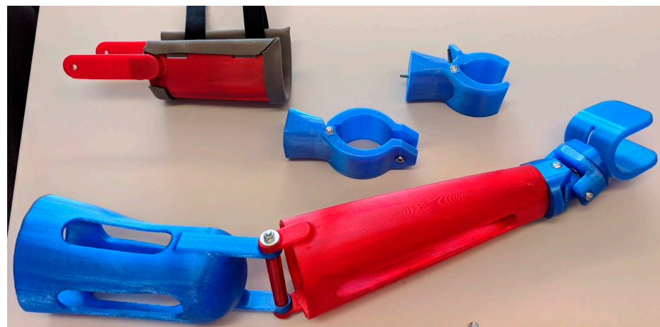
Figure 1. Modular hand prosthesis—basic product considered in the studies, manufactured using Fused Filament Fabrication 3D printing technology, out of PETG material [28].
