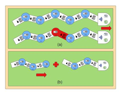
**Figure 4.** Illustrating the benefits of the modular design of the snake robot. This makes it possible to: (a) achieve locomotion even in the event of a module failure; (b) modular reconfiguration (self-assembly) of the snake robot.
