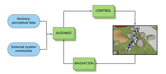
Figure 5. A generalised guidance, navigation, and control architecture for snake robot [65].
