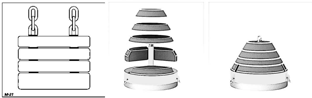
Figure 37 seen from left to right, deadweight steel weights (Vryhof manual, 2015, s. 17) and new type of dead weight design (Offshore wind design AS, 2023)
