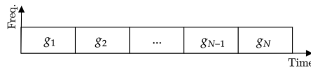
Fig. 1 Groups are assigned to orthogonal resources. The users within a group employ NOMA.
