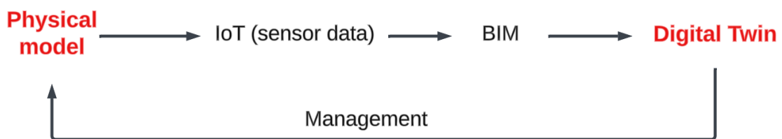
Figure 2.2: Flowchart depicting the relationship between BIM, IoT, and the Digital Twin. BIM and IoT serve as integral components of the Digital Twin concept, with BIM providing a comprehensive digital representation of the physical asset and IoT collecting real-time data.
