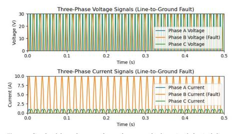
Figure 6. Simulated three-phase waveforms of current and voltage signals for single line-to-ground faults.
