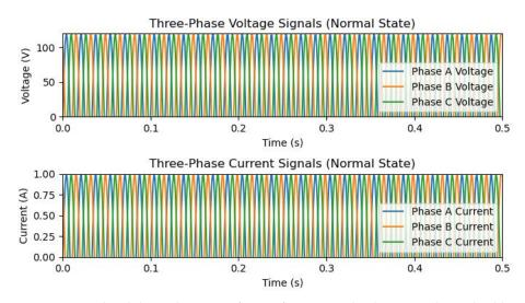
Figure 5. Simulated three-phase waveforms of current and voltage signals in a healthy state.
