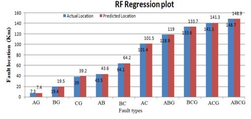
Figure 19. Actual vs. predicted fault locations using Random Forest (RF).
