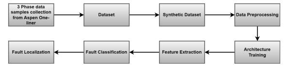
**Figure 2.** An overview of TL Fault Recognition and Localization in power transmission networks using proposed machine learning algorithms.
