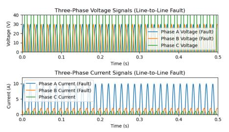
Figure 7. Simulated three-phase waveforms of current and voltage signals for line-to-line faults.
