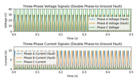
Figure 8. Simulated three-phase waveforms of current and voltage for double phase-to-ground faults.
