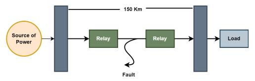
Figure 4. A 220 KV three-phase 150 km transmission network model.
