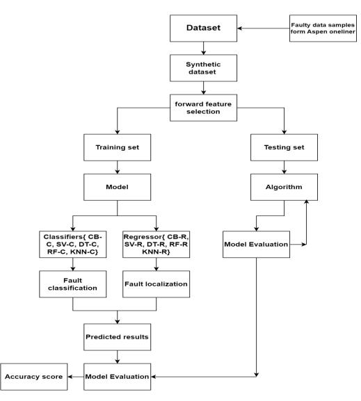
Figure 9. Flowchart of the proposed methodology for fault classification and localization.
