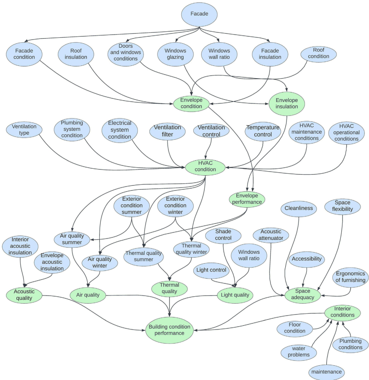
Fig. 5. Graphical representation of the Bayesian Network model for probabilistic evaluation of building comfort performance, after [16].
