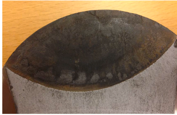
Fig. 10. Cross section cutout of a 145 mm chain link, showing the final crack size after fatigue testing. The crack face is darker due to oxidation.
