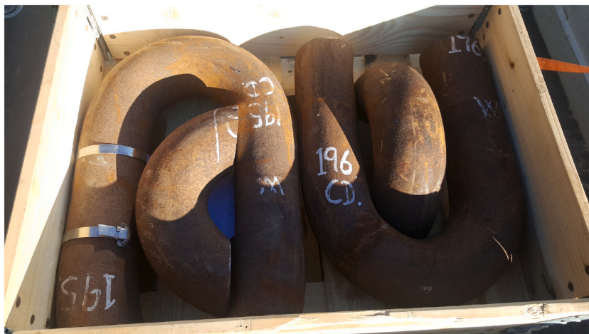
Fig. A.1. Chain links before fabrication of test specimens
