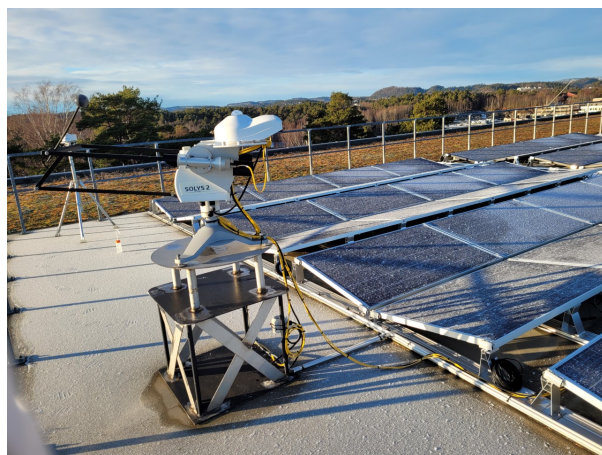
Figure 6.10: Northwest-oriented view of the PV installation on the roof of the University of Agder. GHI, DHI, and DNI pyranometers are installed in the image's foreground. Source [84]
