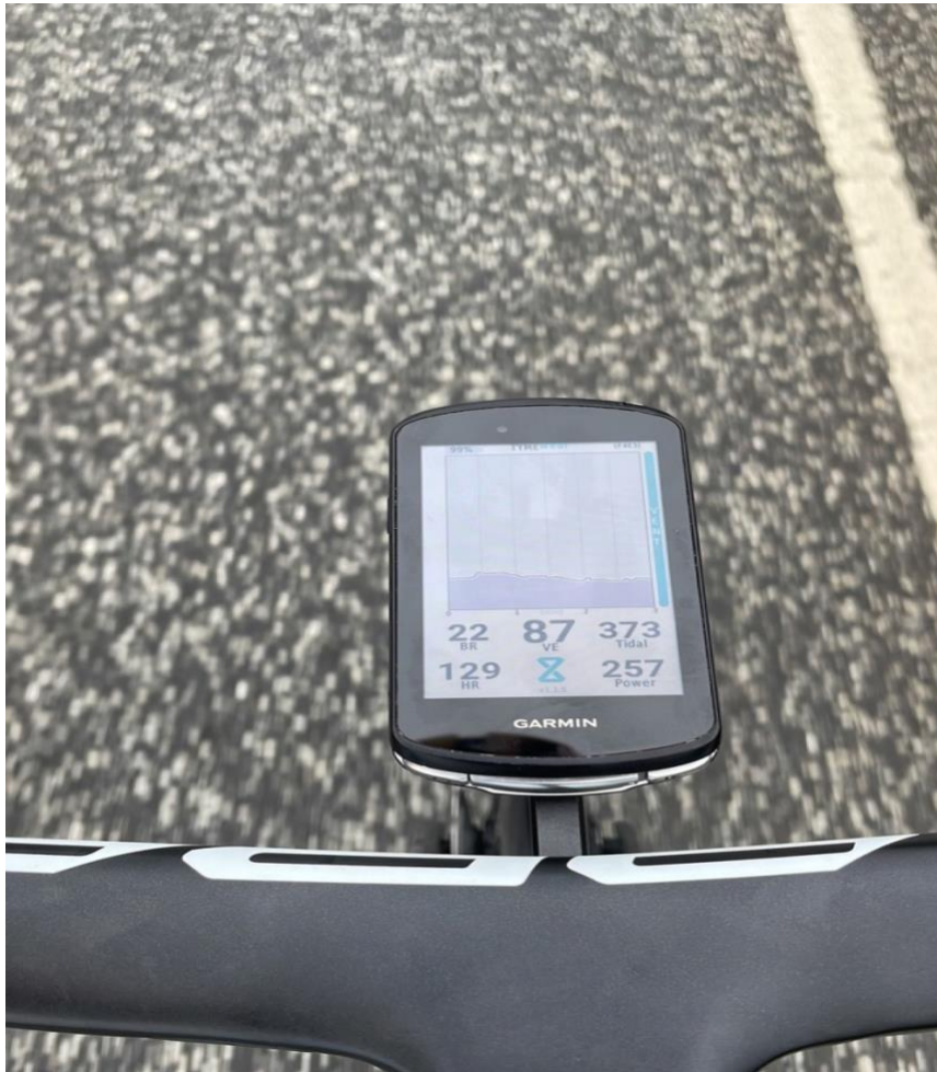
Figure 15: Display of the measurements from the TymeWear smart shirt on a Garmin 1040 cycling computer. Picture from April 2023.
