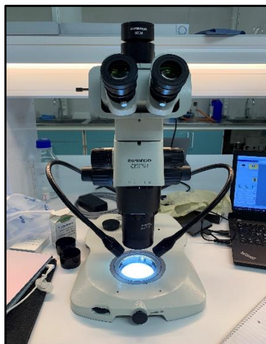
Figure 8. Microscope ( OLYMPUS SZX16 ) with attached camera and analyze software.
