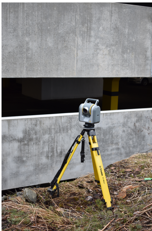
Figur 5.2: Trimble SX12 Scanning Total Station fra SITECH. Foto: Privat
