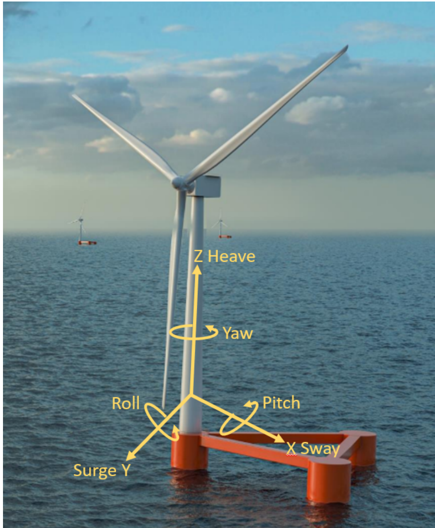
Figure 1.6: Demonstration of six DOF for a FOWT, figure modified from Equinor.
