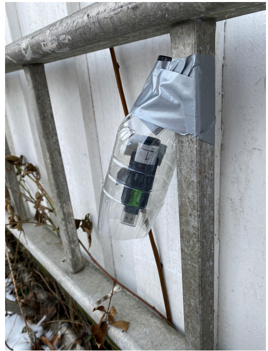
Figure 3.15: Rain Protected Outdoor Logger
