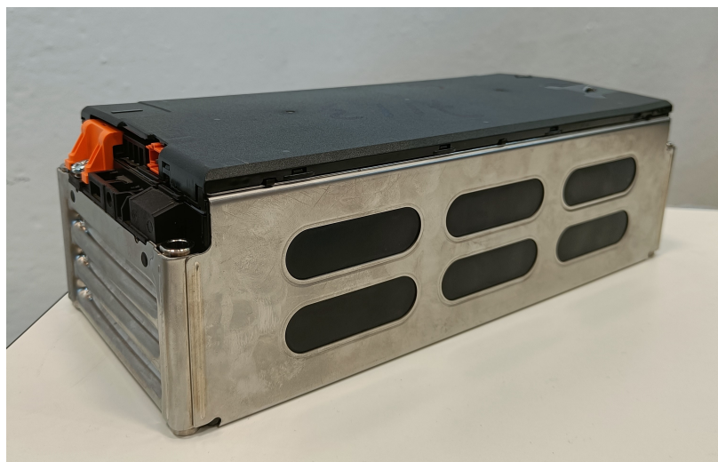
Figure 3.1: VW e-Golf battery module
