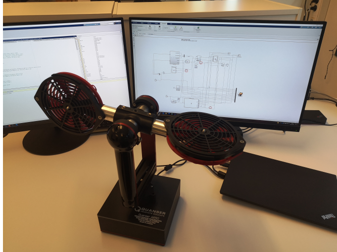
Figure F.5: Quanser Aero helicopter system connected with computer.
