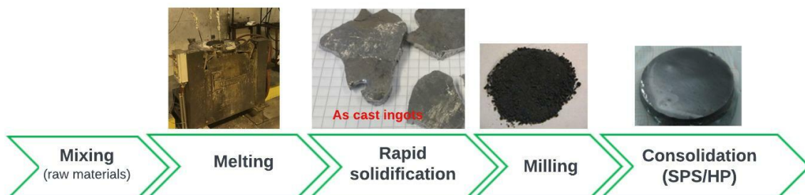
Figure 2.5: Overview of the conventional melting and pouring synthesis method and further material processing from the as cast ingots
