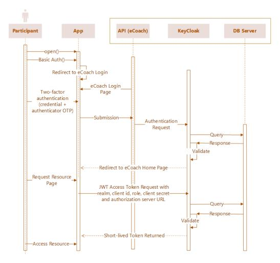
**Figure 7.** Sequence diagram of the login process for accessing web resources following the SSK security solution.
