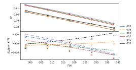
(d) FF and  $\beta^r_{\rm FF}$  as a function of the cell temperature.
