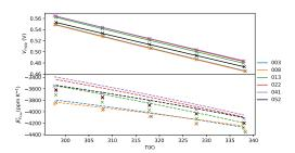
(a)  $V_{\rm mpp}$  and  $\beta^r_{V_{\rm mpp}}$  as a function of the cell temperature.
