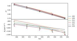
(d) FF (top) and  $\beta_{\text{FF}}^r$  (bottom) as a function of the cell temperature.
