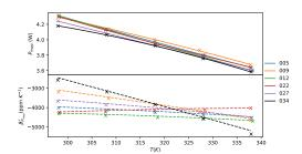
(b)  $P_{\rm mpp}$  (top) and  $\beta^r_{P_{\rm mpp}}$  (bottom) as a function of the cell temperature.
