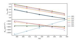
(b)  $P_{\rm mpp}$  and  $\beta^r_{P_{\rm mpp}}$  as a function of the cell temperature.
