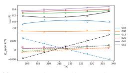
(c)  $i_{\text{mpp}}$  and  $\beta^r_{i_{\text{mpp}}}$  as a function of the cell temperature.
