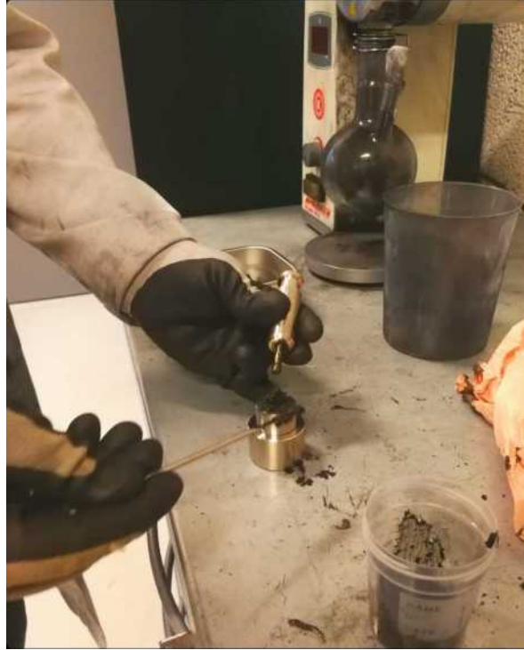
Figure 16: Agglomeration pellet method
