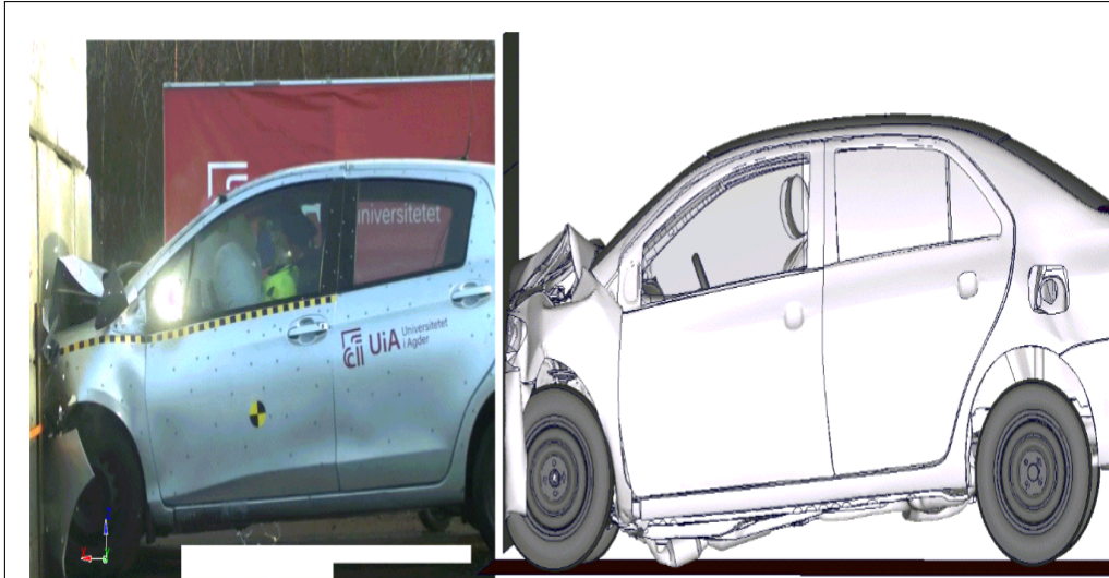
Figure G.21: Physical Test vs FE comparison for full scale test in side view
