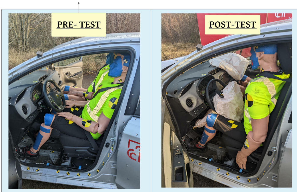
Figure G.17: Test vehicle in Side View with Dummies and Airbag Deployment - pre and post impact.
