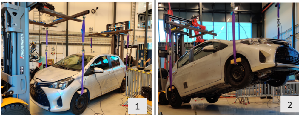
Figure G.7: CG measurement; 1) Measurement of forces without tilting the vehicle; 2) Tilting vehicle front by 30 degrees
