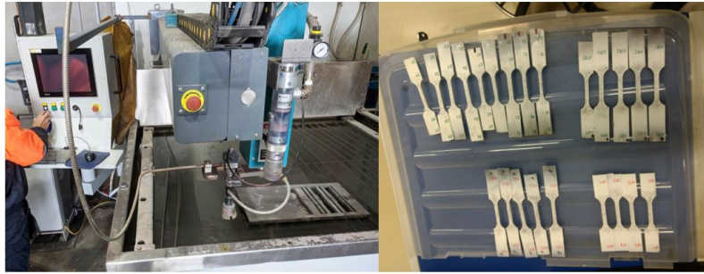
Figure F.4: Water jet cutting of the samples, dog-bone samples
