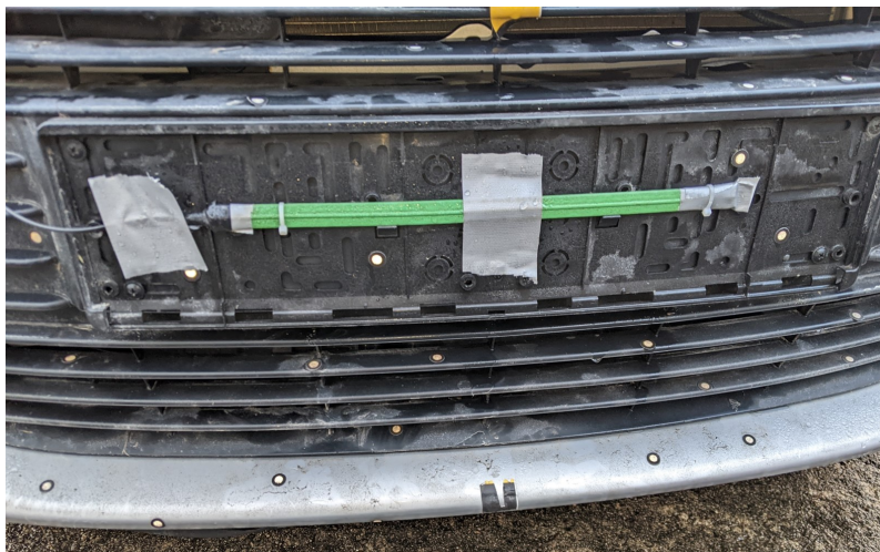
Figure G.11: Contact based trigger mounted on the vehicle.
