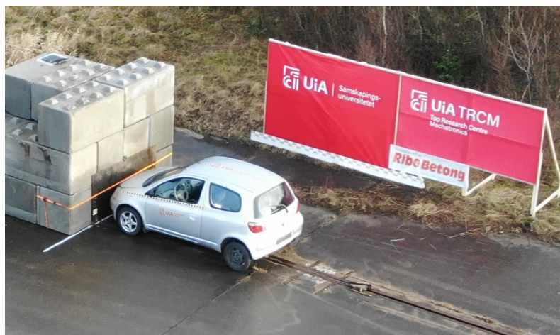
Figure G.8: Concrete barrier used in the test.
