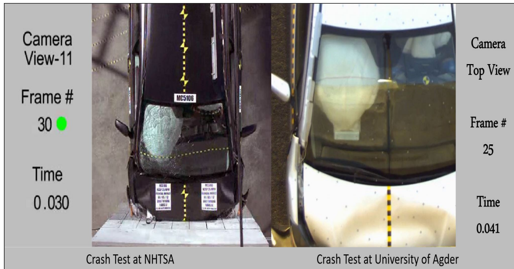
Figure G.20: Airbag deployment timings compared NHTSA vs Crash test at UiA - close to end of deployment
