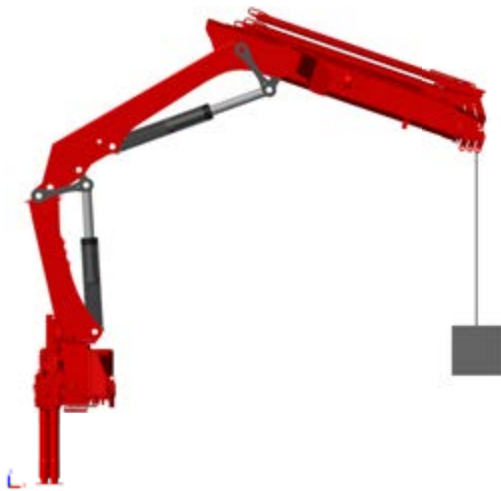
Figure 7: 2D view of the crane model in MATLAB Simscape™.
