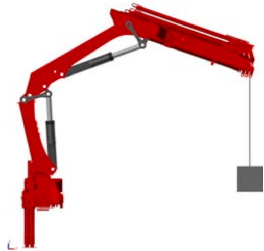
Fig. 7. 2D view of the crane model in MATLAB Simscape™.
