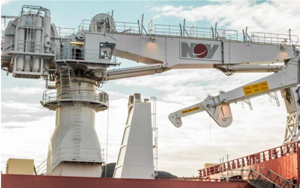
Figure 1.1: Typical offshore knuckle boom crane shown in resting position, manufactured by National Oilwell Varco [1]. Taken from Paper A.
