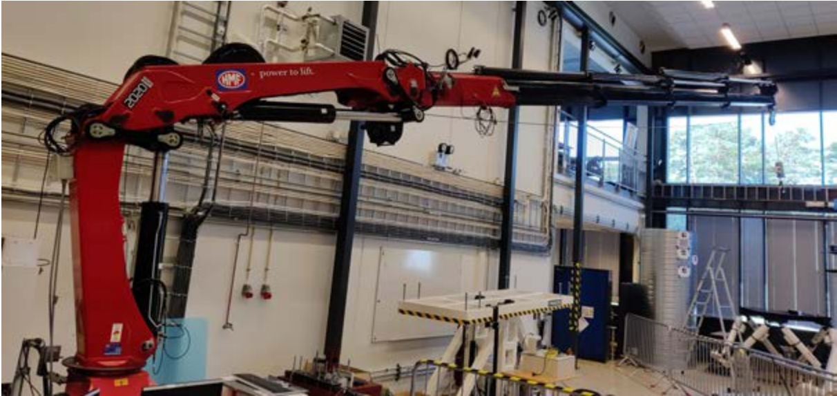
Figure 1.2: The HMF 2020K4 crane in the laboratory with the telescopic booms extended.
