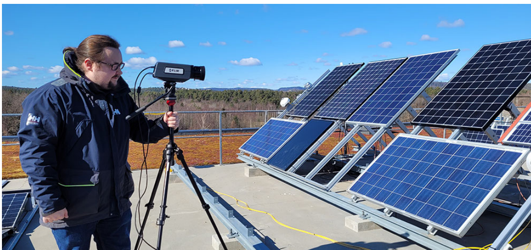
Figure 4.6.1: Photography of the author with FLIR A6750 MWIR camera on tripod, set up for infrared thermography imaging of photovoltaic modules.
