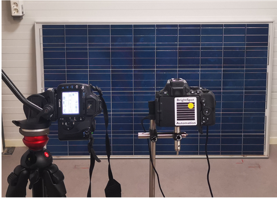
(a) Camera setup for ultraviolet fluorescence imaging- (left), and electroluminescence imaging (right) experiments.
