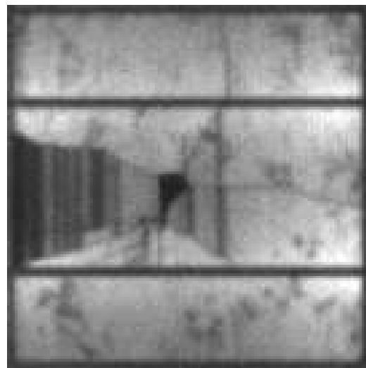
Finger fault type B, faulty finger connections caused by cell-cracks.
