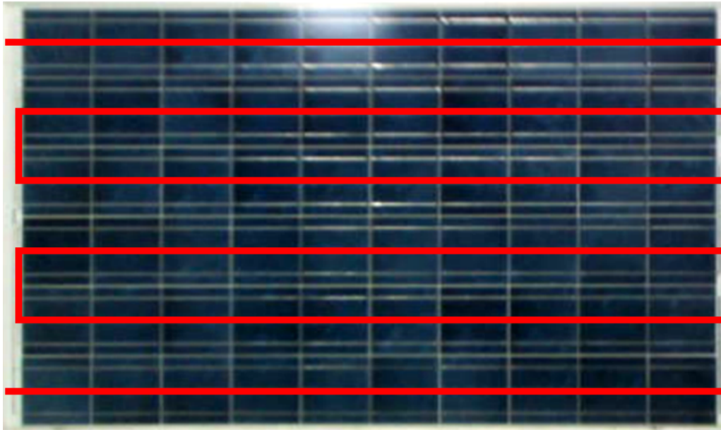
Figure 5.5.1: Photography of module with designation \beta -I, with circuit diagram overlay. Bypass-configuration unknown.
