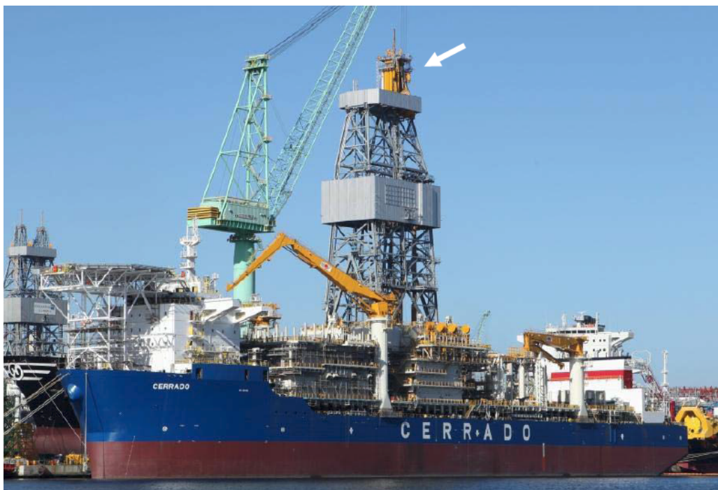
Figure 2.2: CMC location on top of the derrick of the Cerrado drillship
