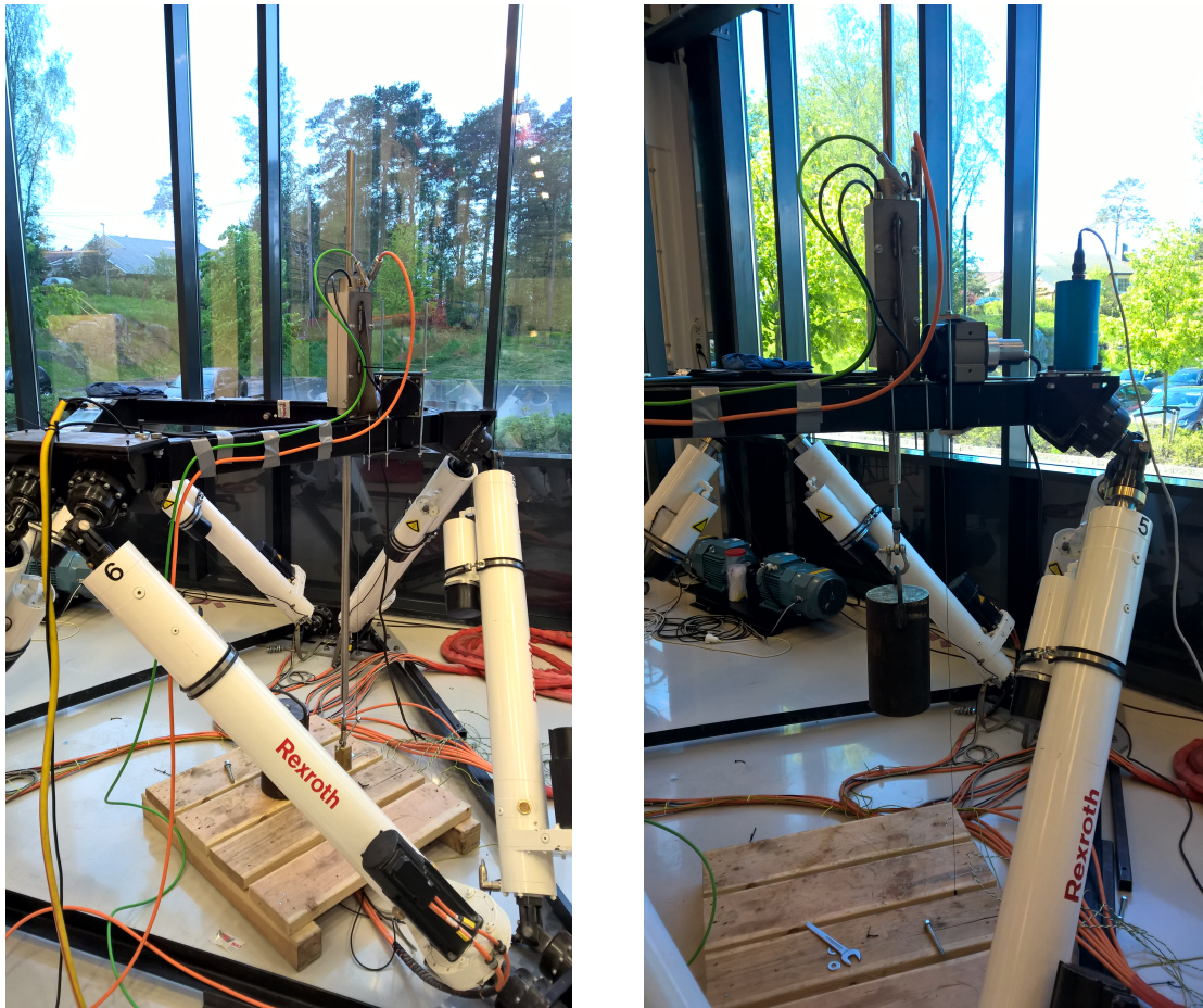
(a) The linear motor AHC test setup
