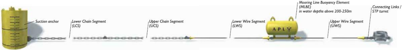
Figure 2.2: Flexible mooring system (National Oilwell Varco, 2014d, pp. 4-5).
