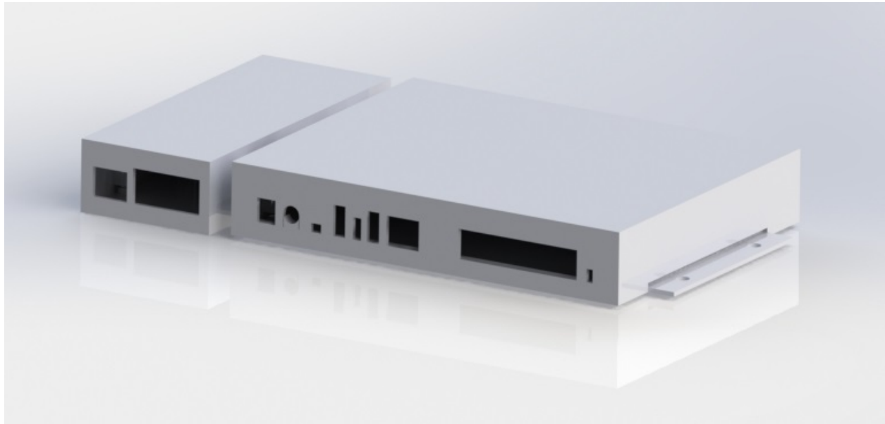
Figure 3.9: Assembled box of both TP-link and Raspberry Pi.
