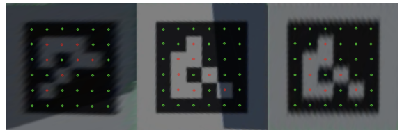
(d) Keypoints detected (Stage-2), number of markers on screenshot 59 with brightness -50%.
