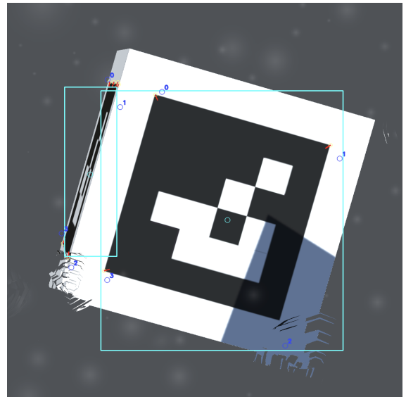
(b) Detection of boxes and corners (Stage-1) in screenshot 51 with rain drops in the image.
