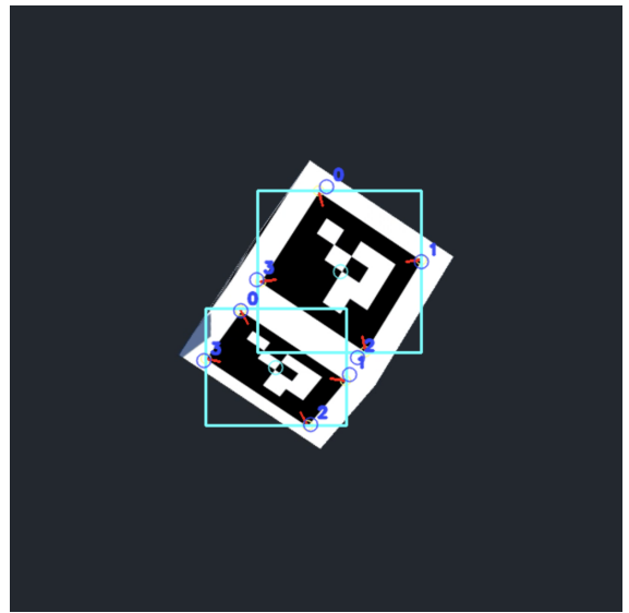
(b) Detection of boxes and corners (Stage-1) in screenshot 90 with contrast increased to 90%.
