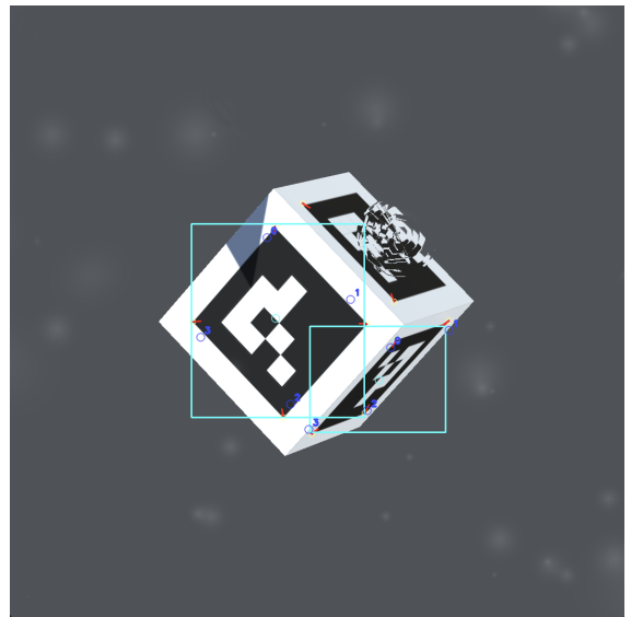
(b) Detection of boxes and corners (Stage-1) in screenshot 41 with rain drops in the image.
