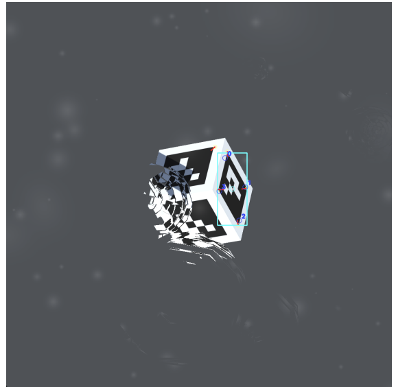
(b) Detection of boxes and corners (Stage-1) in screenshot 3 with rain drops in the image.
