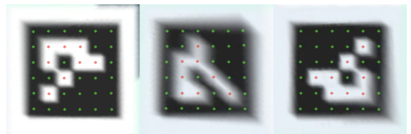
(d) Keypoints detected (Stage-2), number of markers on screenshot 3 with motion blur.
