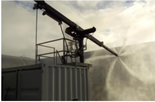
Figure 3.7: The robotic high pressure lance for daily cleaning [73]
