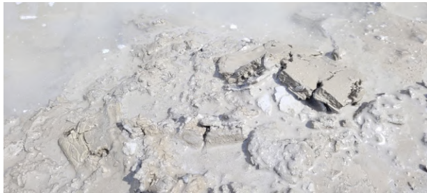
(a) Wet CS that has sedimented and then is shovelled up again. The wastewater can be seen in the top left
