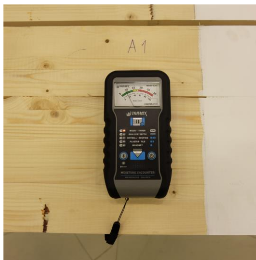
Figure 6.7: Tramex moisture content encounter
