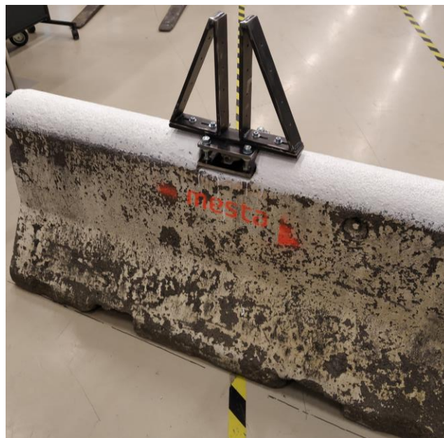
Figure 6.2: Support boundary with a frictionless steel bracket working as a lateral restraint.
