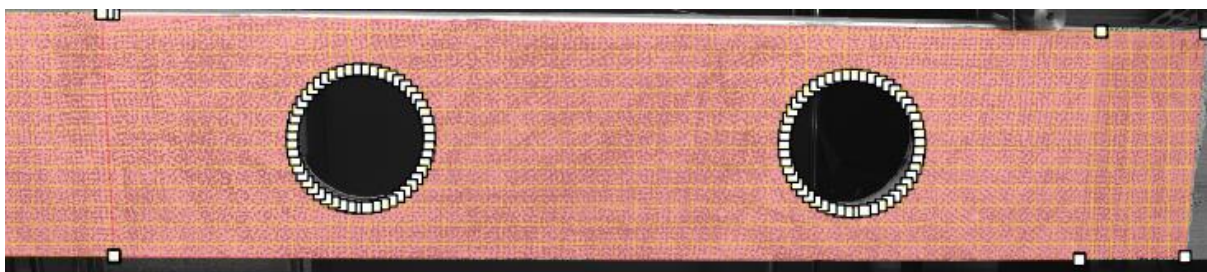
Figure 6.12: Defined area of interest with a cutout around the hole area. This example is from specimen B1.
