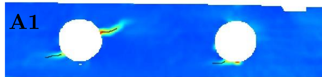
Figure 12.1: ACDM crack contour plot of specimen A1 before complete failure
