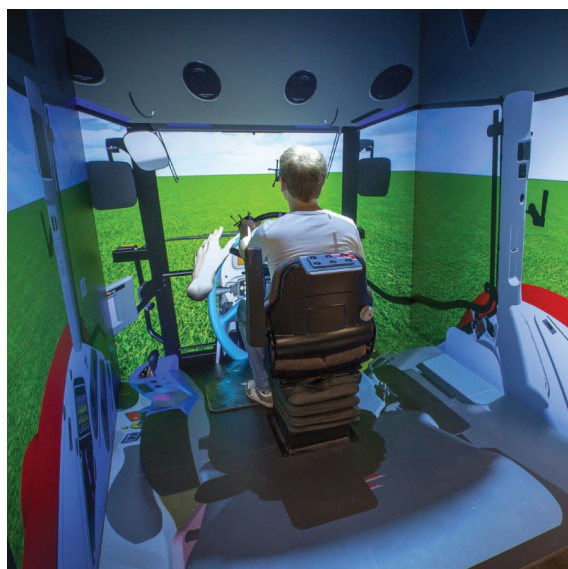
Figure 2.3: CAVE simulation immerses the user with a set of displays that surrounds the user [36]
