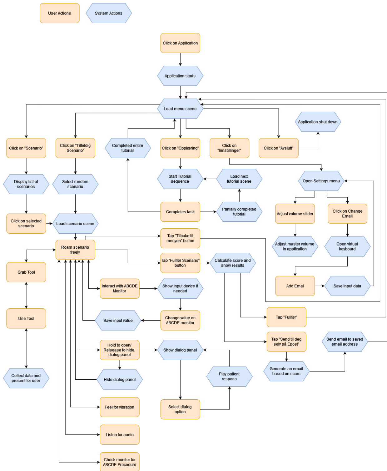
Figure 3.8: Simplified conceptual model of the application (See appendix E for full version).
