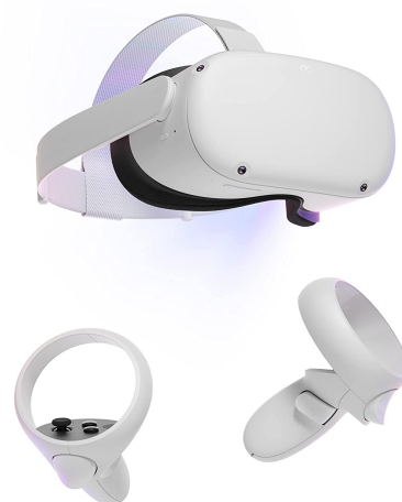
Figure 2.4: Meta Quest 2 is a HMD that immerses the users by placing a stereoscopic display close to the eyes of the user [37]
