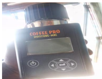
Figure 5. 8 Coffee moisture meter
