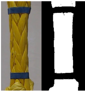
Figure 7. Areas with markers (left) and the binary image after HSV conversion and thresholding (right).
