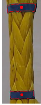
Figure 6. Measurement area with mid points of markers. The distance between these points are used for length measurements.
