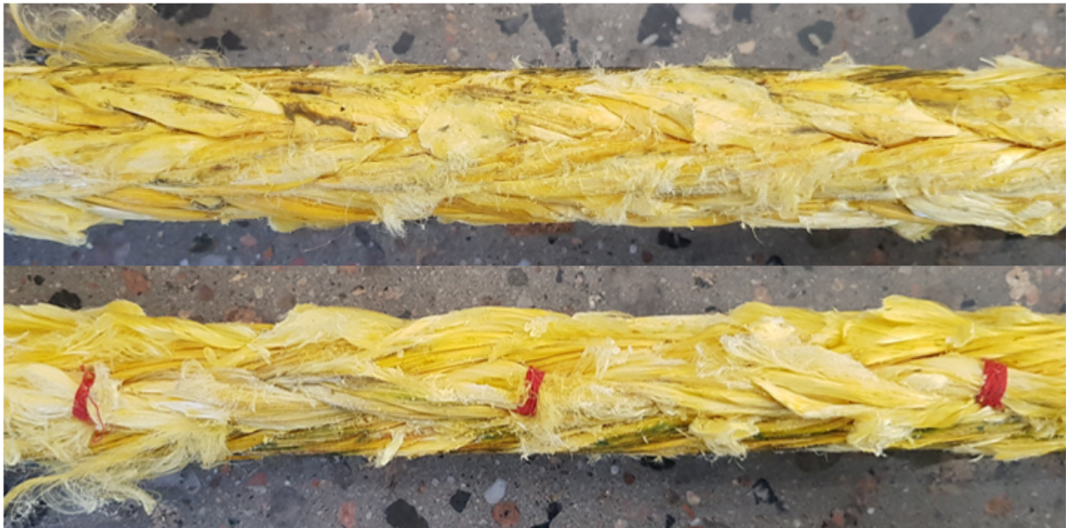
Figure C.8: Compression damage (top) and extruded loops (bottom).
