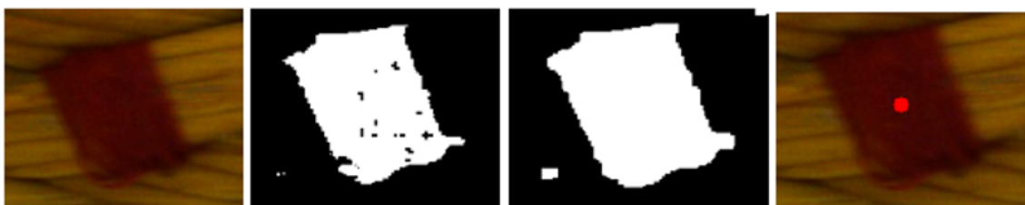
Figure C.4: Different stages and effects of morphological operations applied to the image to detect a specific colour for length measurements: (a) original image, (b) binary image created, (c) dilation operation applied and (d) final processed image with centre point of marker visible after contouring operation.
