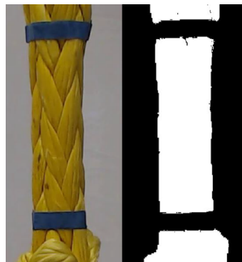
Figure A.7: Areas with markers (left) and the binary image after HSV conversion and thresholding (right).
