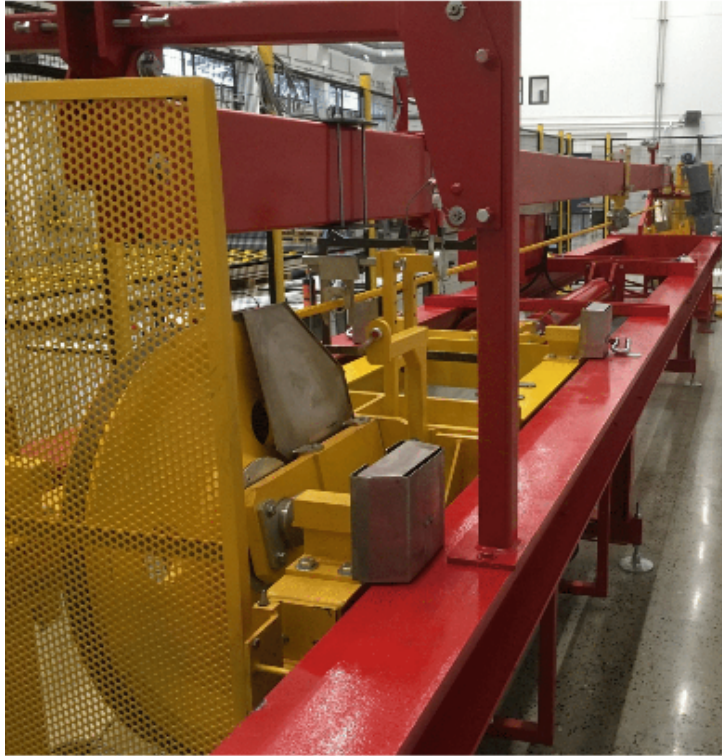
Figure C.1: CBOS test machine as located the MIL, Norway. View is from just behind the test sheave with the driving sheave visible at the far end of the test frame.
