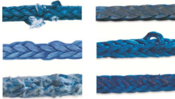
Figure A.1: Different kinds of rope damages. Cut strands (top left), compression damage (top right), inconsistent diameter (middle left) and pulled strands (middle right), heavy abrasion (bottom left) and melted fibers (bottom right). Reproduced with permission from Samson Rope Technologies.
