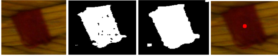
Figure B.4: Elongation algorithm process (left to right): (a) original image, (b) binary image based on colour mask, (c) dilation and (d) processed image with centre point found based on contouring.
