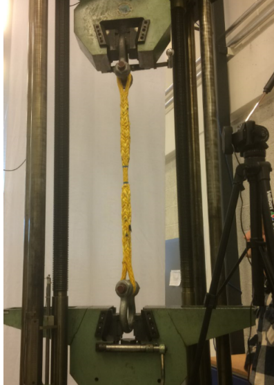
Figure A.4: Experimental set up. Here a fiber rope is secured into the tensioner.
