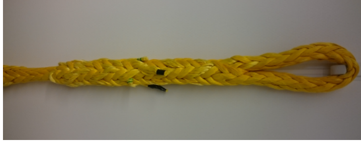
(a) An example of the splice used for the ropes during tension testing.
