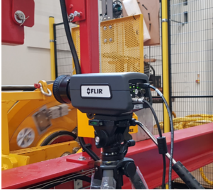
Figure 3.5: View of FLIR A6753sc infrared thermal camera during CBOS testing for steel wire ropes.
