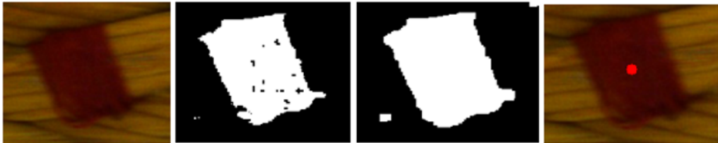
Figure 4.1: Morphological operations applied to the image to detect a specific colour for length measurements: (a) original image, (b) binary image created, (c) dilation operation applied and (d) final processed image with centre point of marker visible after contouring operation.
