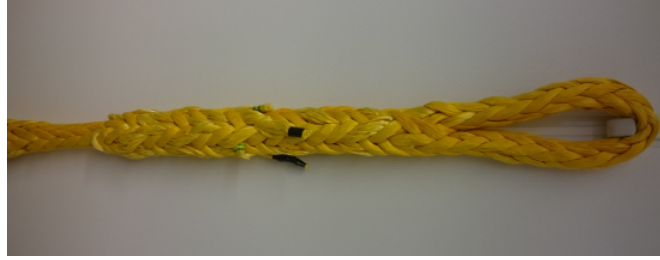
Figure A.2: Example of splice and eyelet at the end of a fiber rope specimen.
