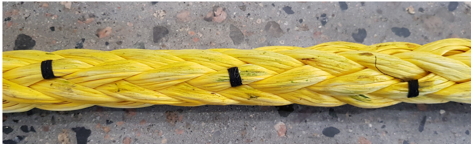
(b) Example of threads sown into a rope sample to designate a bending zone.
