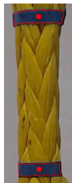
Figure A.6: Measurement area with mid points of markers. The distance between these points are used for length measurements.
