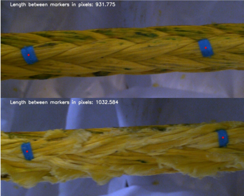
Figure 4.8: Example of increase in local length in the DBZ from the start (top) and end (bottom) of a CBOS test.
