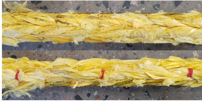
Figure 4.5: Compression damage (top) and extruded loops (bottom).
