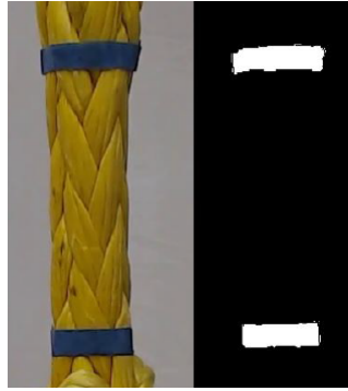
Figure A.5: Area with markers (left) and the binary image after HSV conversion and thresholding (right).
