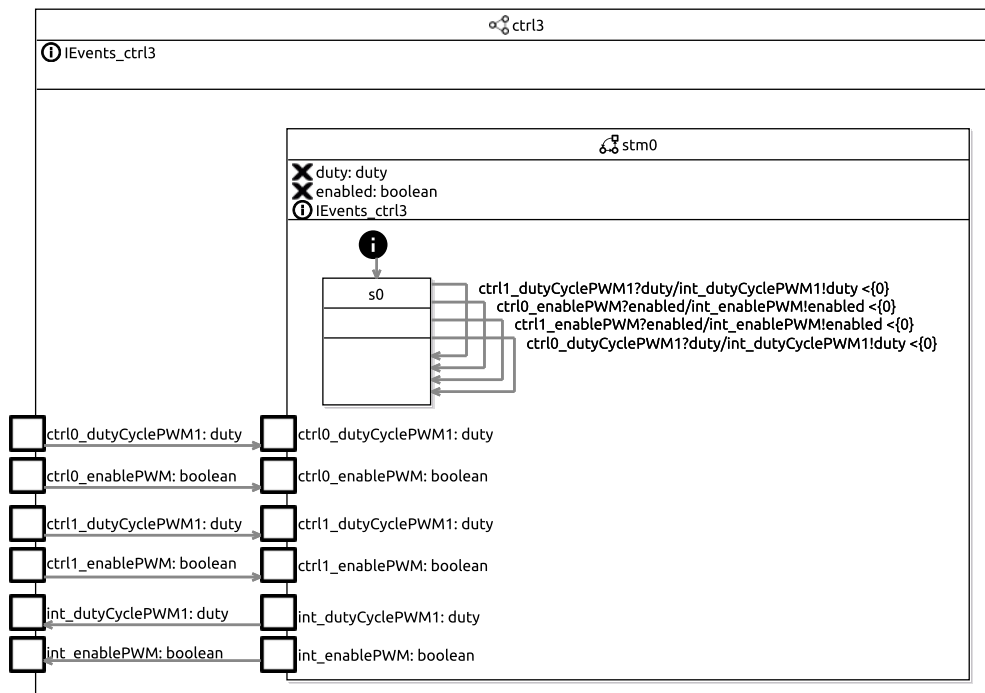
Figure A.21: Controller ctrl3 with state machine stm0 that relays input events from ctrl0_dutyCyclePWM1, ctrl0_enablePWM, and ctrl1_dutyCyclePWM1 and ctrl1_enablePWM, through int_dutyCyclePWM1 and int_enablePWM.
