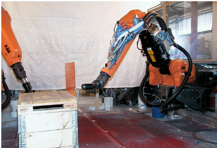
Figure 4: Setup for experimental testing with paint using ABB robot. Photo courtesy ABB, from [5].
