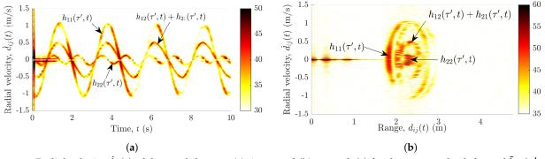
**Figure 2.** Radial velocity  $\dot{d}_{ij}(t)$  of the pendulum vs. (a) time *t* and (b) range  $d_{ij}(t)$  for the measured subchannel  $\tilde{h}_{22}(\tau', t)$ .
