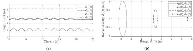
**Figure 9.** (a) The analytical radial range components  $d_{ij}(t)$  and (b) the analytical radial velocity components  $\dot{d}_{ij}(t)$  for  $(L_1^{T_x}, L_1^{R_x}) \neq (L_2^{T_x}, L_2^{R_x})$ .
