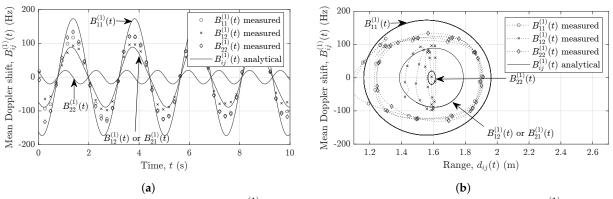
**Figure 10.** (a) The measured mean Doppler shift  $B_{ij}^{(1)}(t)$  vs. time and (b) the measured mean Doppler shift  $B_{ij}^{(1)}(t)$  vs. range  $d_{ij}(t)$ , where the MIMO radar undergoes cross-channel interferences.
