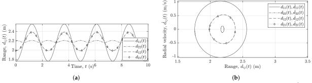
**Figure 8.** (a) The analytical radial range components  $d_{ij}(t)$  and (b) the analytical radial velocity components  $\dot{d}_{ij}(t)$  for  $(L_1^{T_x}, L_1^{R_x}) = (L_2^{T_x}, L_2^{R_x})$ .
