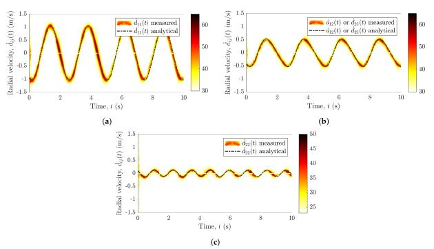
**Figure 6.** Application of the proposed interference mitigation scheme results in segregated measured radial velocity components  $\dot{d}_{ij}(t)$  for the channel links: (a)  $A_1^{T_x} - A_1^{R_x}$  (Radar<sub>1</sub>), (b)  $A_1^{T_x} - A_2^{R_x}$  (or  $A_2^{T_x} - A_1^{R_x}$ ), and (c)  $A_2^{T_x} - A_2^{R_x}$  (Radar<sub>2</sub>).
