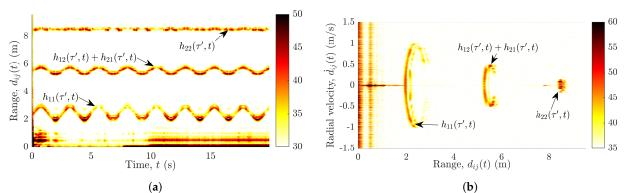
**Figure 5.** Different cable lengths, i.e.,  $(L_1^{T_x}, L_1^{R_x}) \neq (L_2^{T_x}, L_2^{R_x})$ , result in the segregation of (**a**) measured range profiles and (**b**) measured range–velocity profiles.
