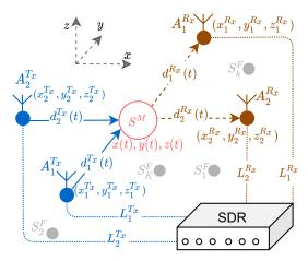
**Figure 3.** Geometrical 3D model for a 2 × 2 MIMO system with a single moving scatterer  $S^M$  and K fixed scatterers  $S^F_k$  (k = 1, 2, ..., K).
