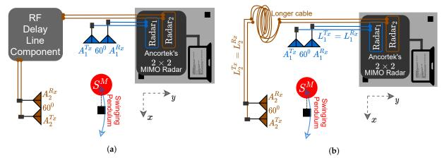
**Figure 4.** Setup to induce a fixed propagation delay by either using (**a**) an RF delay line component or (**b**) different cable lengths, i.e.,  $(L_1^{T_x}, L_1^{R_x}) \neq (L_2^{T_x}, L_2^{R_x})$ .
