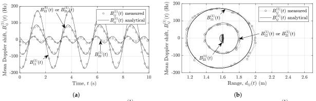
**Figure 11.** (a) The measured mean Doppler shift  $B_{ij}^{(1)}(t)$  vs. time and (b) the measured mean Doppler shift  $B_{ij}^{(1)}(t)$  vs. range  $d_{ii}(t)$ , where the MIMO radar adopts the proposed interference mitigation scheme.
