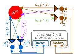
**Figure 1.** Two radar subsystems forming a 2 × 2 MIMO radar system in the presence of a single moving scatterer  $S^M$ .
