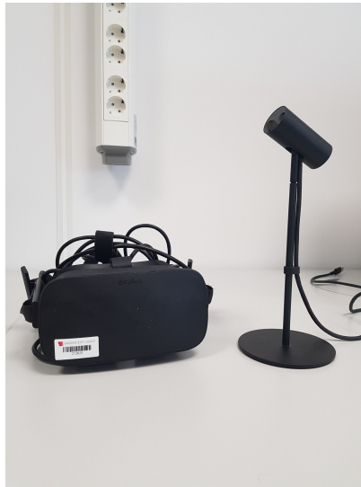
Figure 2.4: The predecessor of the Oculus Rift S. This Oculus Rift uses outside-in tracking technology that tracks infra red signals from the Oculus Sensor.
