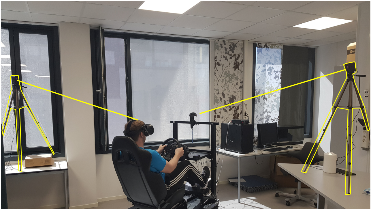
Figure 3.5: The motion platform is flanked on both sides with the lighthouses/base stations. It is important that the lighthouses see each other, the headset and the reference controller fastened on the platform.
